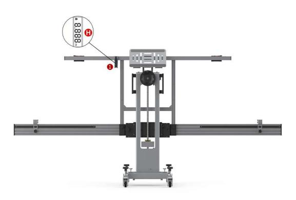
1. Turn on the height range finder ① and adjust the device height so that the value of height range finder ① is H, H=\_\_\_\_mm.
